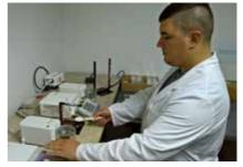
Particle matter sample weighing
